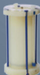
Plastic column for medical protein separation.
