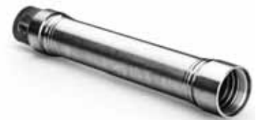
Titanium test cylinder for absorption of crude oil.
