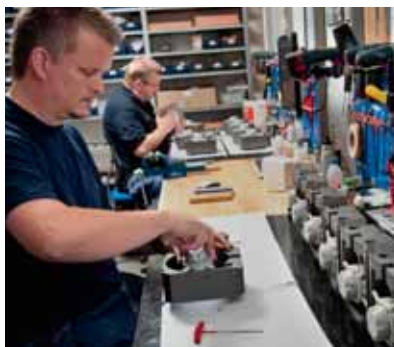
Manual assembly of cardiac pumps at Fredriksons.
