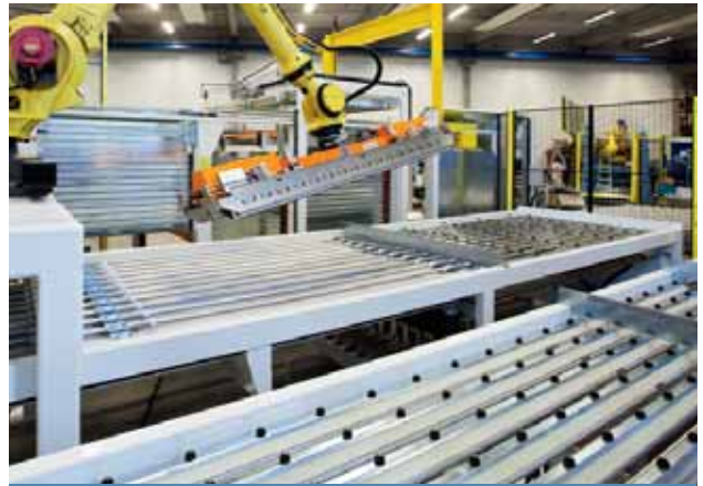
Automated balancing equipment for lids, designed and manufactured by NPB.
