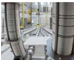
Conveyor system for lids.
