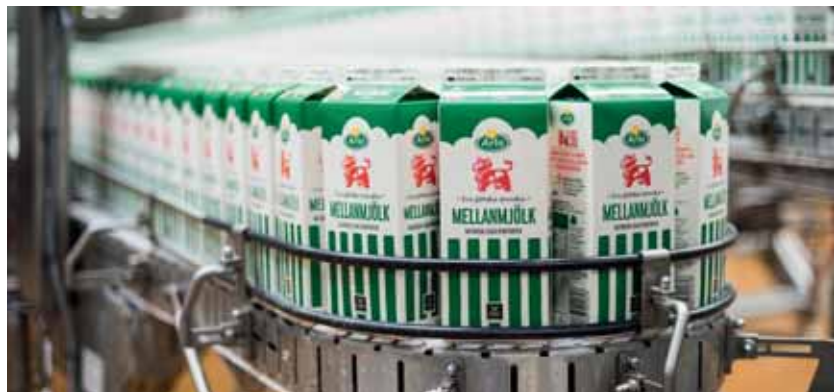
Fredriksons' in-house-developed conveyor system for packaging handling.
