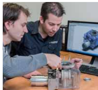
Canline's engineers work with the further development of the company's magnetic brake units for conveyor systems.
