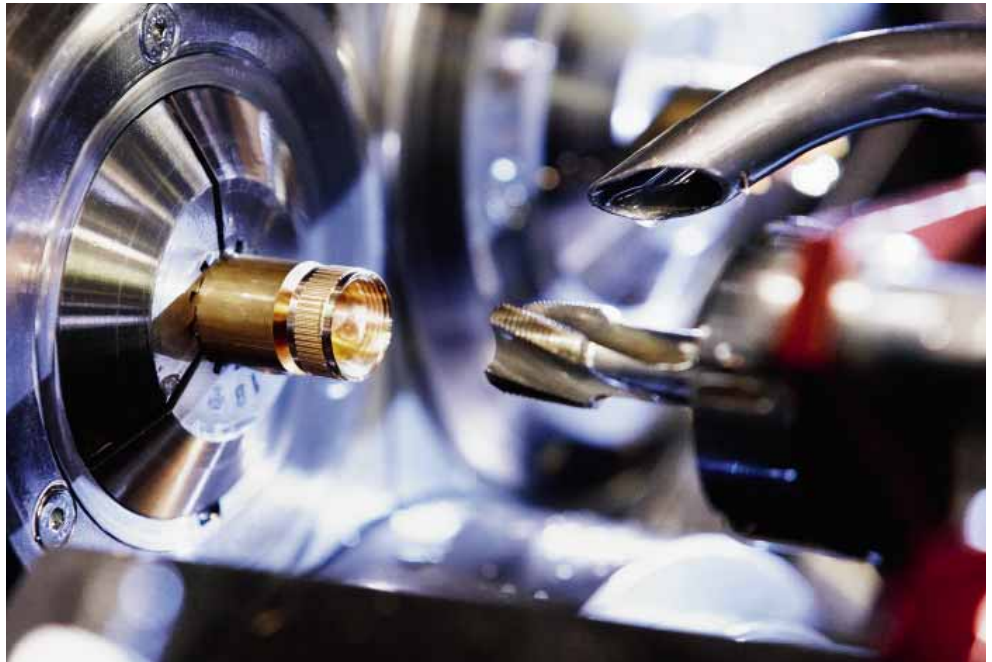
Here a brass component is being turned in a six-spindle automatic lathe.
