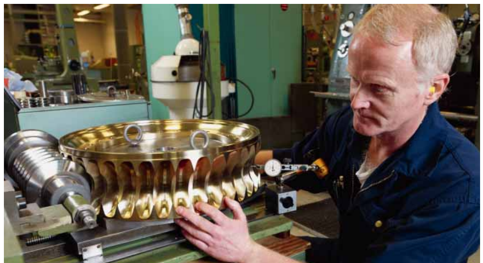
Exact precision is crucial for the customer's end result when manufacturing worm gears at Mikroverktyg.
