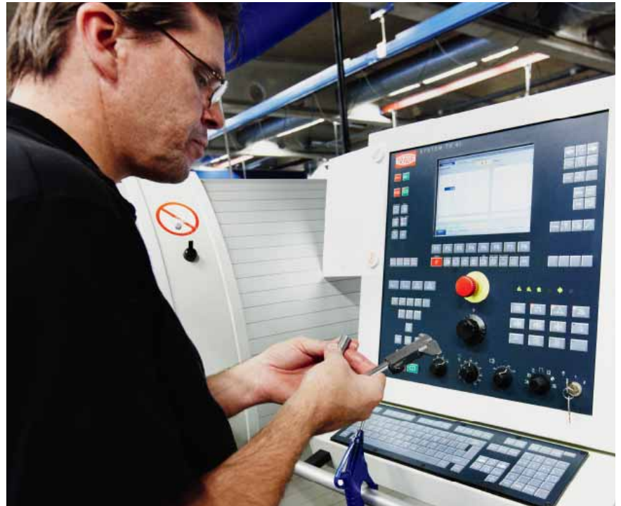
A component is surveyed before production start in a CNC-operated longitudinal lathe at Segerströms.
