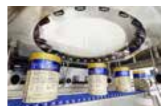
Integrated optical scanner for checking cans in the production line.
