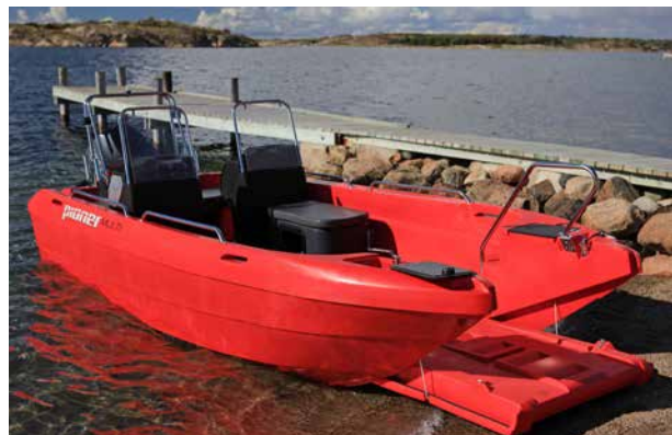
Cipax's Pioneer Multi boat is rotational moulded in one piece and the catamaran-like hull provides excellent sea-keeping qualities. The wide, folding bow door further enhances user-friendliness.
