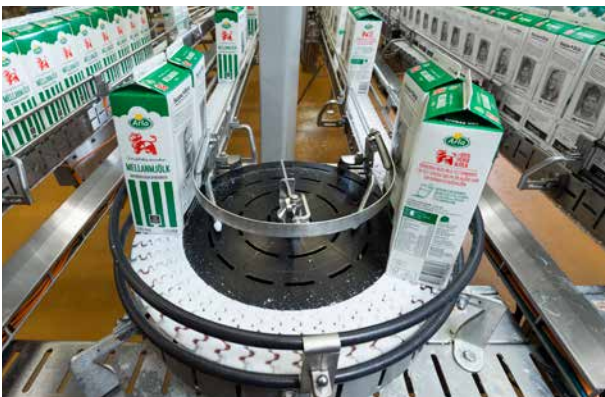
Fredriksons' conveyor system for handling packaging. The equipment includes both conveyor and handling systems, as well as control and software solutions.
