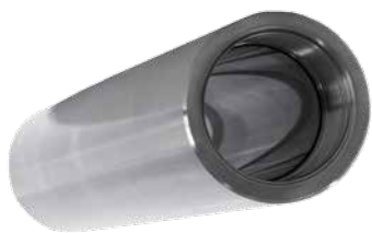
Titanium test cylinder for absorption of crude oil.
