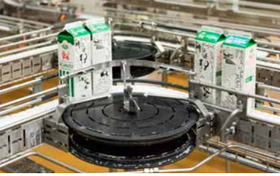
Conveyor system for dairy products.
